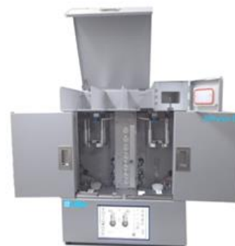
Achieva-CS high-density, large-scale stem cell culture device
